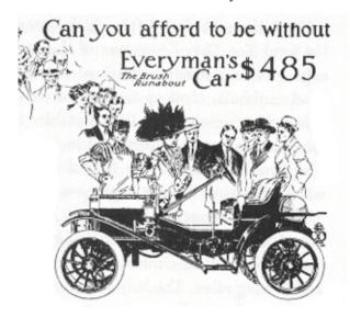
The 1911 Brush had a wooden frame and axles, and the engine ran "backwards" (counterclockwise). The coil springs were also backwards, acting in tension rather than compression.
